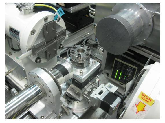
A setup under development at HXMA to measure x-ray absorption spectroscopy under high pressure. The setup has adapters to accommodate several types of diamond anvil cells (DACs). Users supply the DACs. Combined XAFS and x-ray diffraction measurement capability is planned.
